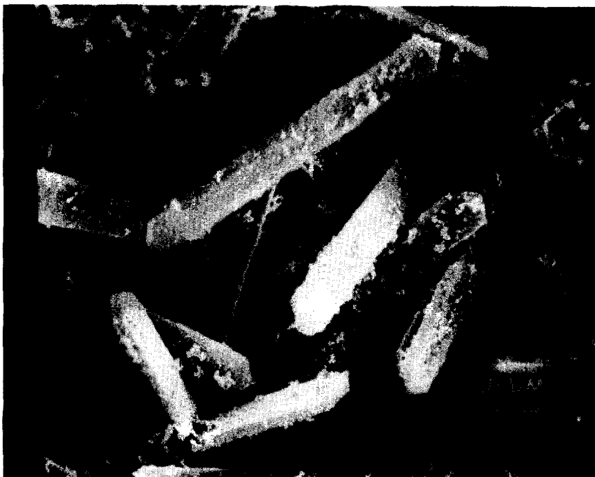
FIG. 9. Scanning electron photomicrograph of the coexisting "harmotome-like" and ZSM-5 phases.
