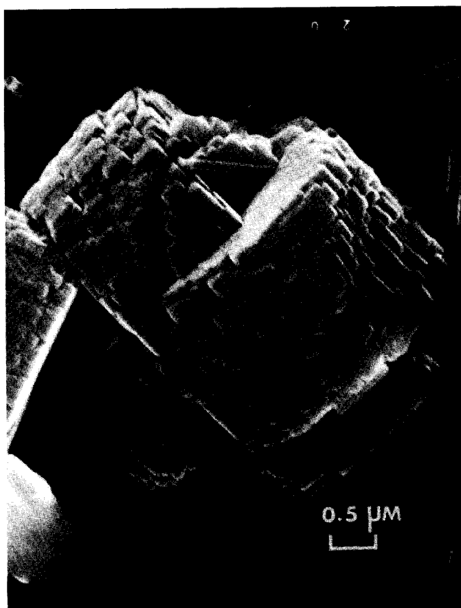
FIG. 8. Scanning electron photomicrograph of K-ZSM-5 crystals from a reaction mixture with the ratio K/(K + TPA) = 0.2 .
